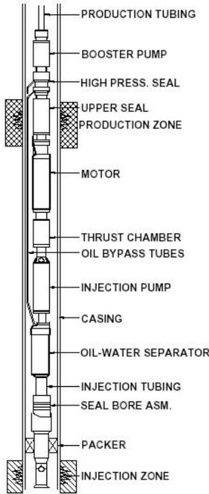
**Figure 1 Schematic drawing of a Hydrocyclone Oil/Water Separator**
