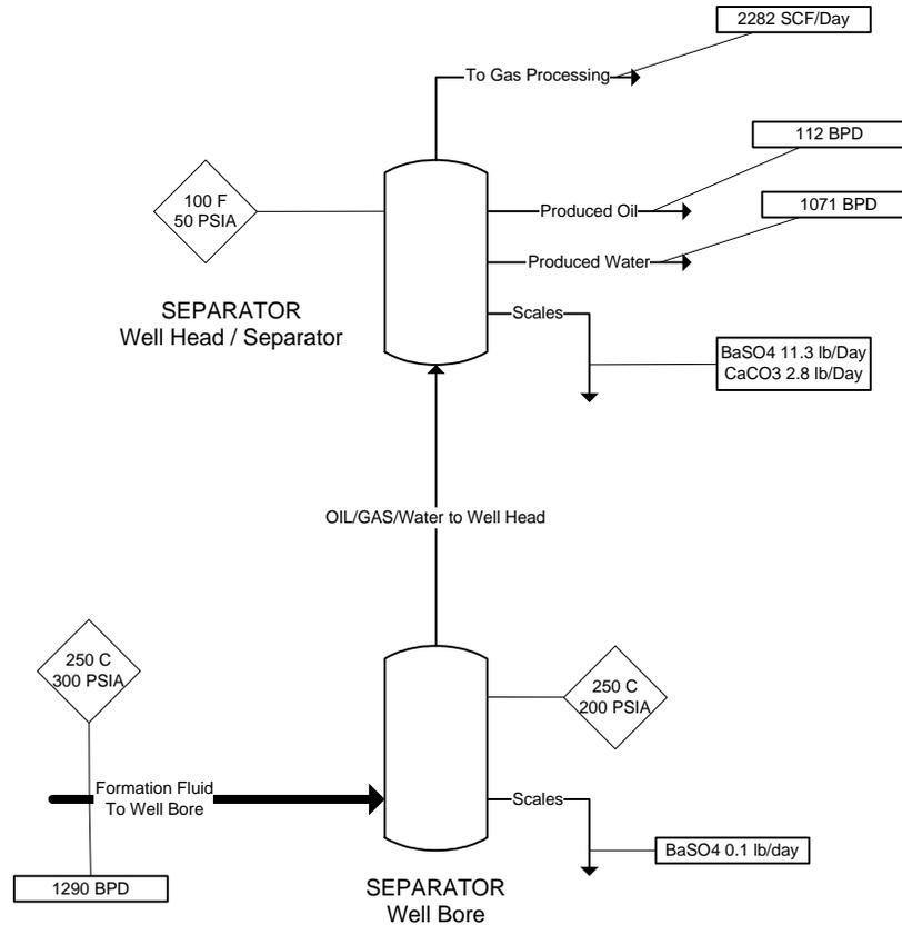
**Figure 2 Non-DOWS configuration – ESP flowsheet**
