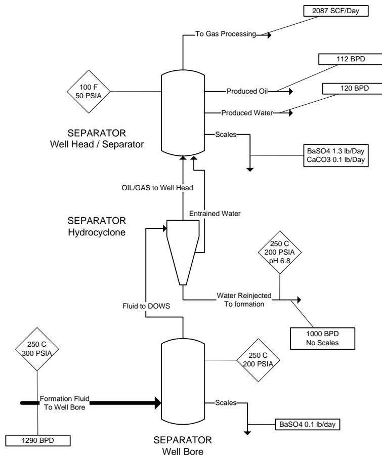
Figure 3 DOWS configuration – ESP flowsheet
